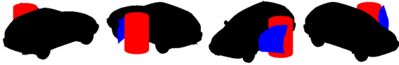
Figure 5: Example occlusion types generated based on the simulation. Representative occlusion types describing relationships among human, door, and vehicle body are presented.
