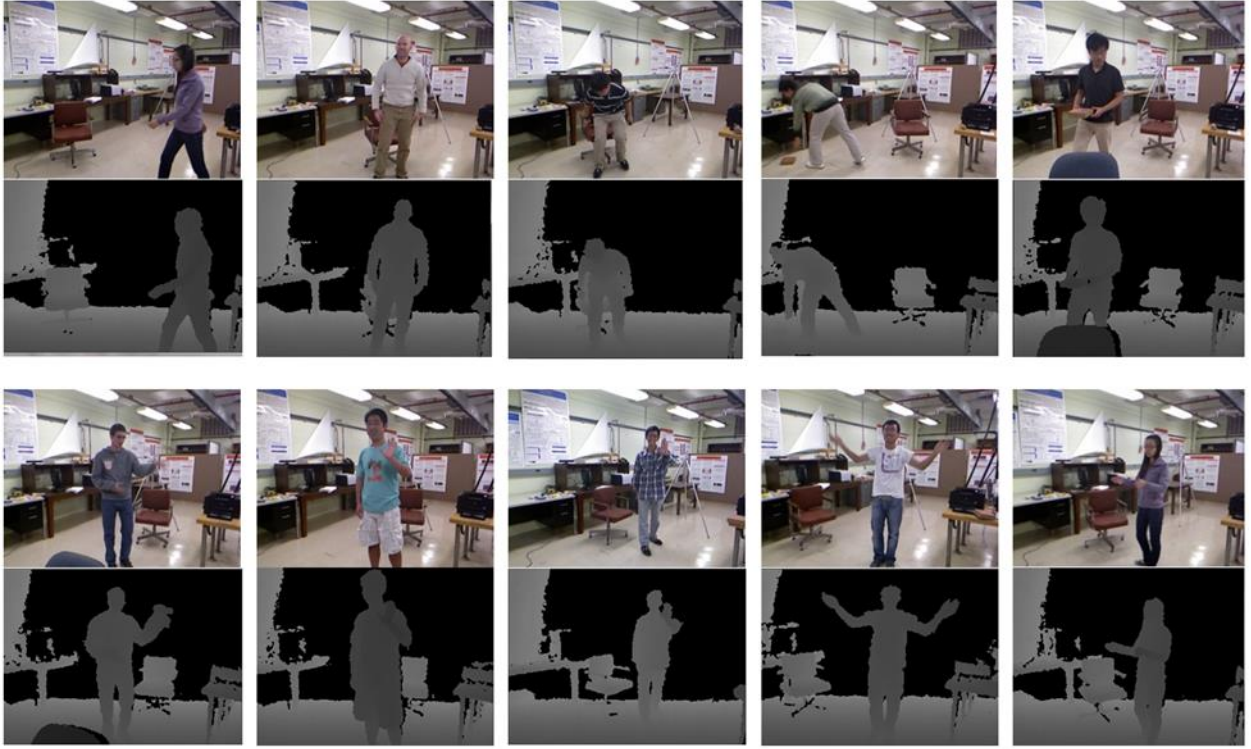
Figure 6: Sample images from videos of the 10 activities in our database. We show RGB image frames as well as the corresponding depth maps. Note only depth images are used in the algorithm. Action type from left to right, top to bottom: walk , stand up , sit down , pick up , carry , throw , push , pull , wave hands , clap hands .
