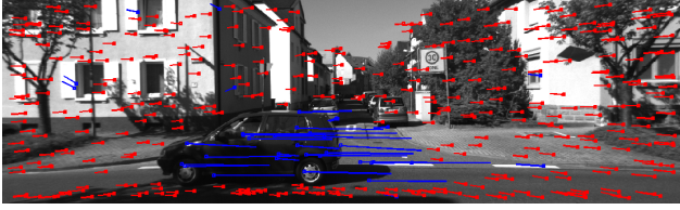
Figure 4: Feature correspondences are classified into inliers (red) and outliers (blue) in outlier rejection. This image is from KITTI dataset (No. 7, 729th frame).
